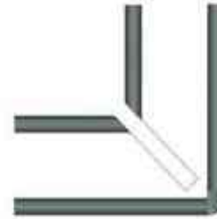
V-shaped 90° Groove if folded up to 90°
