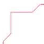
STD. OUTSIDE CORNER TRIM AT INTERSECTION OF END WALL & SIDEWALL
