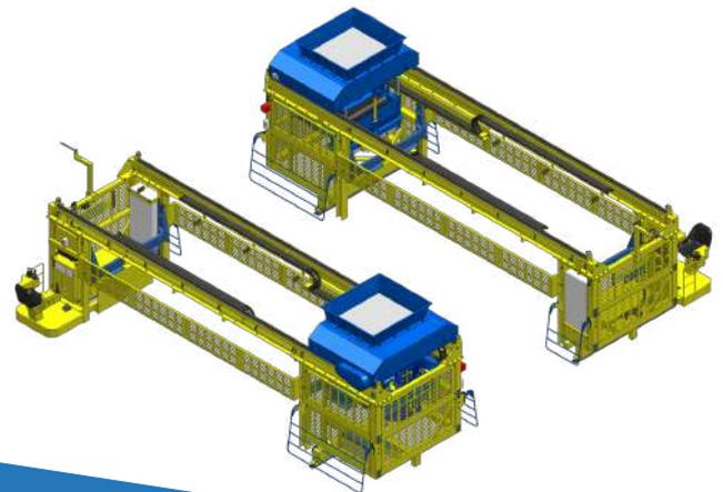
This machine carries out a complete dry cast process, it uses a belt feed and hopper for fast filling, powerful linear vibration and employs a unique rotary screeding process.
