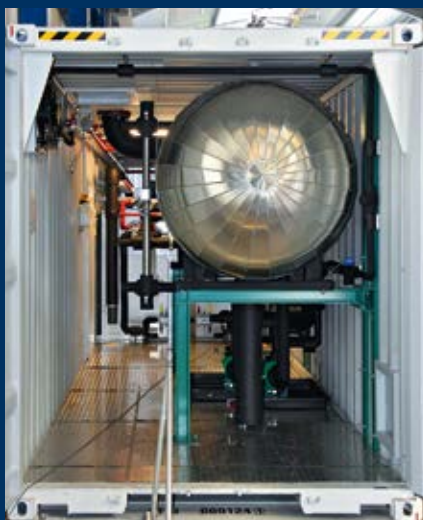
Ammonia separator with ammonia pump
