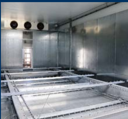
Ice storage with rake system
