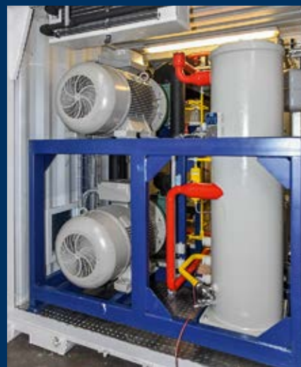
Open-type screw compressors with oil separator
