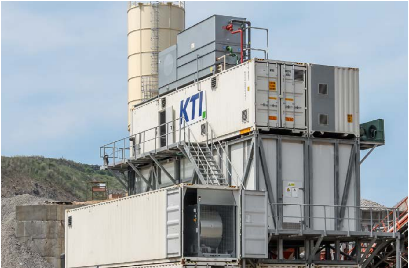
2x PLIP 100 on top of MIS 75 and Cold Water Plant beside
