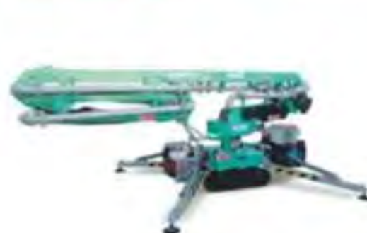
Gerris 800 Crawler Concrete Placing Beam Self propelled machine with reduced dimensions (300 x 400 mm) and low weight (2500 kg). Ideal for distributed concrete in any position within its range of action of about 8 m and up to a height of 11.20 m. Double motorization: gasoline (main) and electric (auxiliary).
